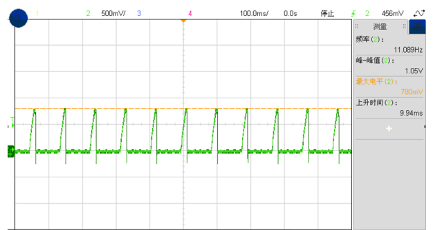
Figure 9, Short circuit & Out voltage
