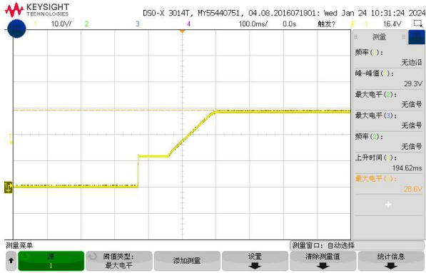
Figure 6, Output voltage established (Iout = 50A)
