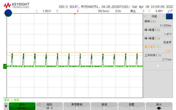
Figure 9, Short-circuit & Output voltage (Iout = 60A)
