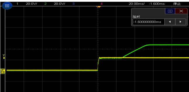
Figure 6, Output voltage established (Iout = 10A)
