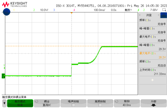
Figure 6, Output voltage established (Iout = 15A)
