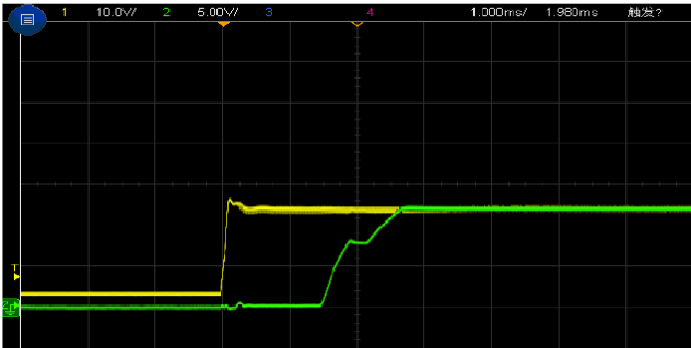
Figure 6, Output voltage established (Iout = 5A)
