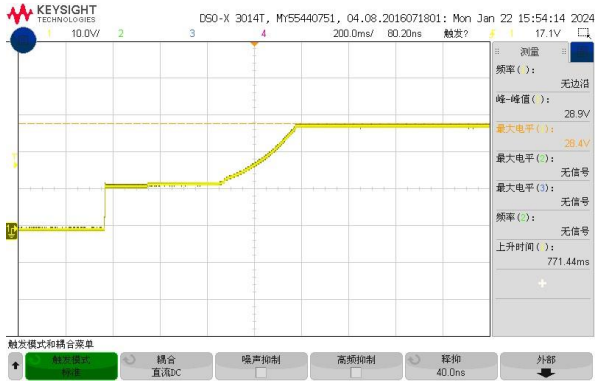
Figure 6, Output voltage established (Iout = 30A)
