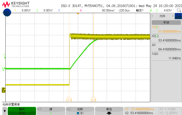
Figure 8, Boot delay time (Iout = 60A)
