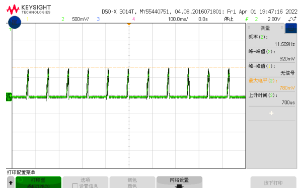
Figure 9, Short-circuit & Output voltage (Iout = 60A)
