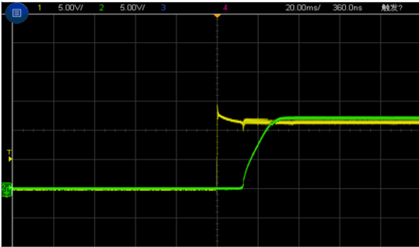
Figure 6, Output voltage established (Iout = 20A)
