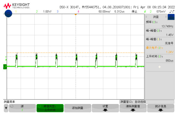
Figure 9, Short-circuit & Output voltage (Iout = 60A)
