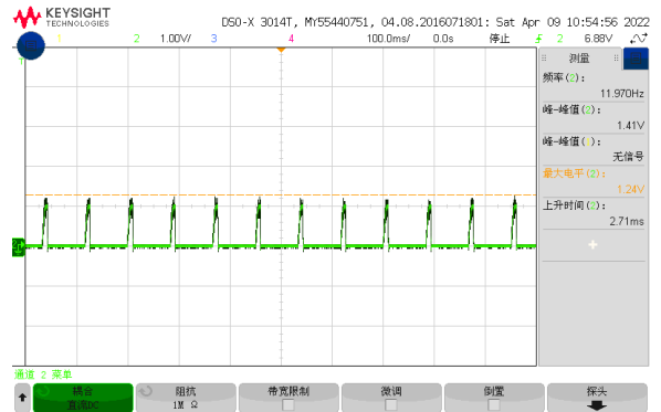
Figure 9, Short-circuit & Output voltage (Iout = 50A)
