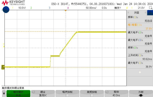
Figure 6, Output voltage established (Iout = 30A)
